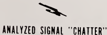
Figure 9. A distorted support plate signal and the processed non-flaw resultant signal. Tracings of actual field data.
