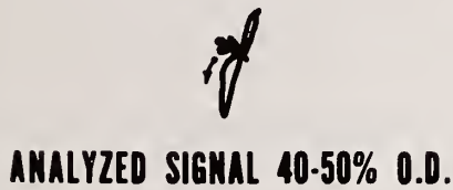
Figure 7. A distorted tube support plate signal and the resultant flaw signal after subtracting a good support plate reference signal. Tracings of actual field data.
